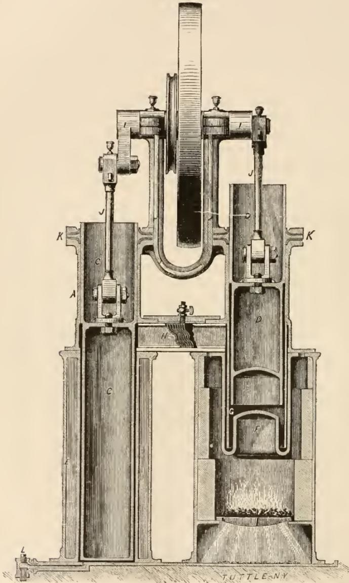
to ascend, the plunger comes down and the operation is repeated. When the air passes from the heater to the cool cylinder A, it heats the plates of the regenerator and this heat is given off to the cool air, when it is again forced into the heater. The utmost of the heat is thus utilized that is possible. The start in this as in all hot-air and gas
